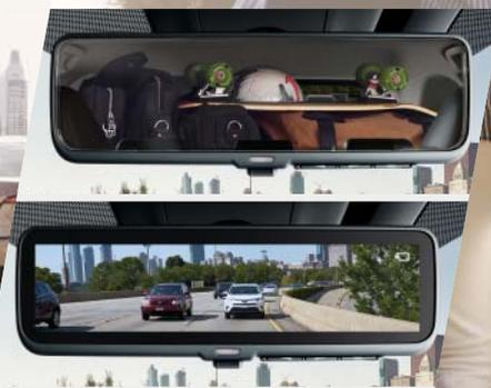
*The new digital rear-view mirror gives drivers a better view of their surroundings. At the touch of a button, the electrochromatic auto-dimming mirror becomes a high-definition digital monitor. And because it uses a camera mounted high up on the RAV4's back window, the monitor always ensures a clear view, even when obscuring items are stored in the boot.*
